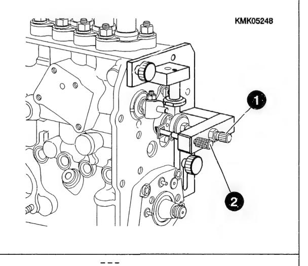
Checking position of RPS shortcircuiting ring: It must be possible to insert the measuring rod without resistance even if the control rod is turned and released again.
